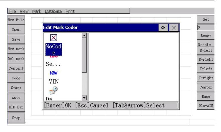
Because we want to make the tag content for fixed content, which means they do not need to change in the imprint is finished, so here we will use the default "no code". Click again on the top right corner of the window (OK) button, appeared engraving engraving control software operating area in the tag we established, as shown below:
