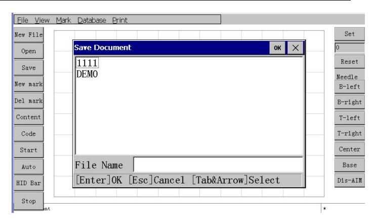
"Save" Window lists all the files in the development of engraving machine, enter a file name in the "file name" column, and then click the top right corner of the window (OK) button or press (Enter) key, the file is saved.
