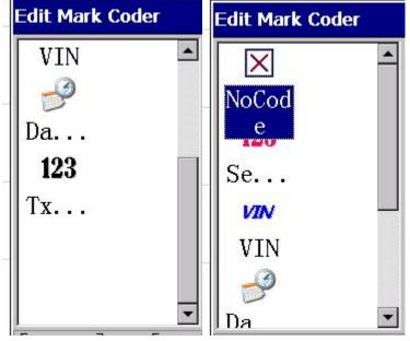
a. The NoCod: As the name suggests, the non-coding means that the content of this tag does not require an engraving after the completion of each change, so this code there is no argument.
