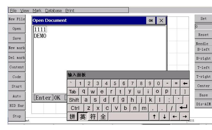
"Open " window that lists all the files in the development of engraving machine, choose one, click on the upper right corner of the window (OK) button or press (Enter) key, the file is opened.
