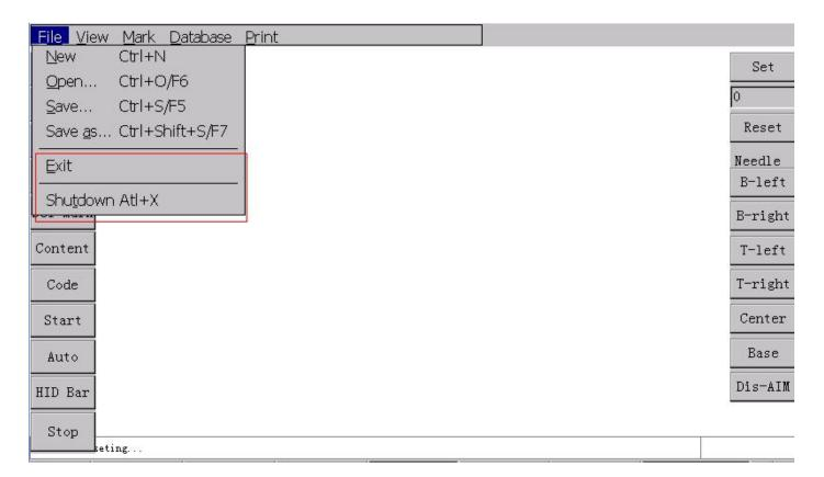
exit: Exit the engraving control software, returning integrated machine main interface.
